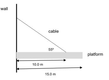
The platform is designed to support a load of 8.5 tonnes and is 15 m long. A single steel cable supports the platform, attached 10.0 m from the end at 55° as shown in the figure. The platform has a mass of 0.7 tonnes.
