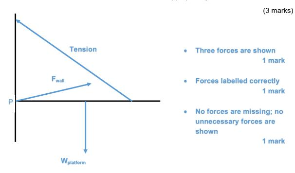
b) Show that with the maximum load acting through the platform's midpoint, the cable will be able to support the platform. Support your answer with calculations.
