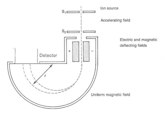
a) Why must the molecules in the vapour be ionized before entering the mass spectrometer?
