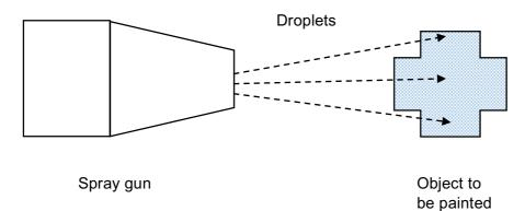
The magnitude of the charge on each droplet is 2.0 x  $10^{-10}$  C and, on average, they have a diameter of about 150  $\mu$ m.
