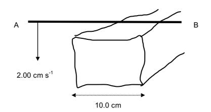
The end of the copper wire marked 'B' gains a net negative charge and the wire generates a small emf with an average value of 2.74 mV.
